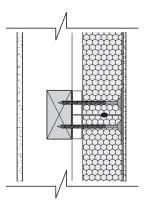
Back blocking required fixed to frame. Vertical panel joints between studs.
